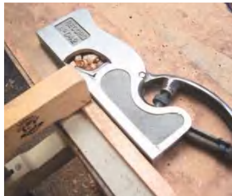
STEP 24. Planing the curve onto the back braces
